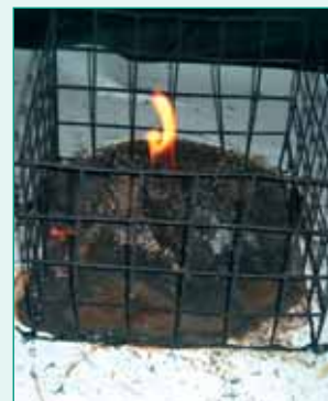
Result of fire test ENV 1187/1.
