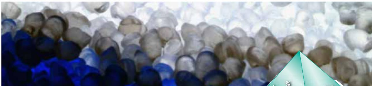
TPE is the collective term for a particular group of polyolefins with the basic properties of elastomers (flexibility, elasticity), but which can be processed as thermoplasts (thermal softening, plastic deformation).
