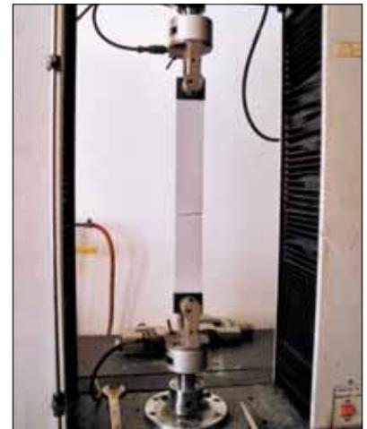
*Spectraplan<sup>®</sup> thermal weld overlap. Weld stronger than the roofing sheet itself.*
